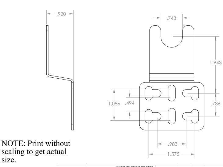
size. UNLESS OTHERWISE SPECIFIED: NAME DATE **O**NEGRill DRAWN DIMENSIONS ARE IN INCHES **TOLERANCES:** TITLE: CHECKED FRACTIONAL± 3PC Bracket ANGULAR: MACH ± BEND ± ENG APPR. TWO PLACE DECIMAL ± THREE PLACE DECIMAL ± MFG APPR. Detail 3 Q.A. INTERPRET GEOMETRIC PROPRIETARY AND CONFIDENTIAL TOLERANCING PER: COMMENTS: THE INFORMATION CONTAINED IN THIS DRAWING IS THE SOLE MATERIAL SIZE DWG. NO. **REV** PROPERTY OF ONEGRILL ANY
