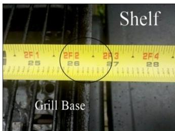
We will round this up to 26 1/2". This is the total width of the part of the grill that houses the burner assembly. It should be taken where the notch for the spit rod is.
