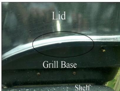
This picture shows the side of a grill. If you notice inside the circled area there are no holes for a bracket. There is also no notch to clear a spit rod. You could drill and notch, but you will lose the protection of the powder coat and it will rust and degrade rapidly.
