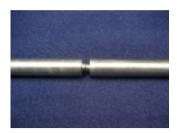
Screw the top post section into the bottom section. The bottom section has a pointed end for penetrating the ground. The top section has a special round feature to help eliminate a mushroom effect of pounding the post into the ground.
