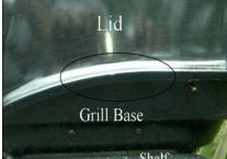
Shelf This picture shows the side of a grill. If you notice inside the circled area there are no holes for a bracket. There is also no notch to clear a spit rod. You could drill and notch, but you will lose the protection of the powder coat and it will rust and degrade rapidly.
