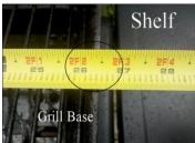
We will round this up to 26 ½". This is the total width of the part of the grill that houses the burner assembly. It should be taken where the notch for the spit rod is.
